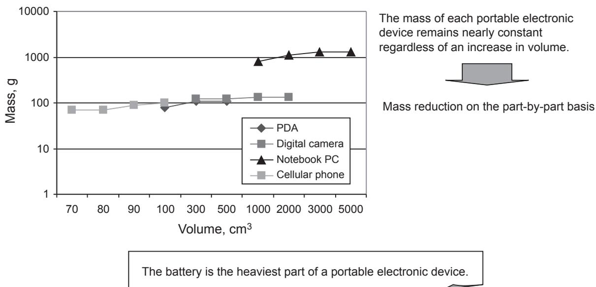
Fig. 2 Volume vs. Weight - Portable Electronic Devices (Survey in FY2000)
