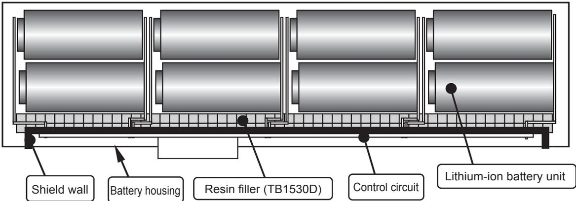
Fig. 6 Lithium-Ion Battery Leakage Prevention System
