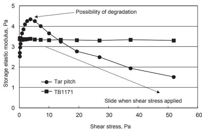
Fig. 5 Comparison of Sealants - Thermal Elastic Modulus (Heating Temperature: 260°C; Frequency: 1 Hz)
