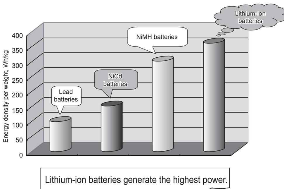
Fig. 1 Comparison - Energy Densities of Secondary Batteries
