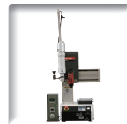
Cartridge-type tank (TC2) Dispensing valve (HPNV-50) Controller for pressure (coater S4) Desktop robot (RT8 Series)
